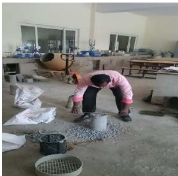
Bulk density test of coarse aggregate
